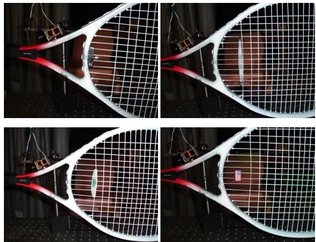
FIG. 6. (Color online) The vibration dampers attached to the racket (electromagnet vibration method shown, but not employed): (a) Babolat model, (b) Head model, (c) Prince model, and (d) Wilson model.
